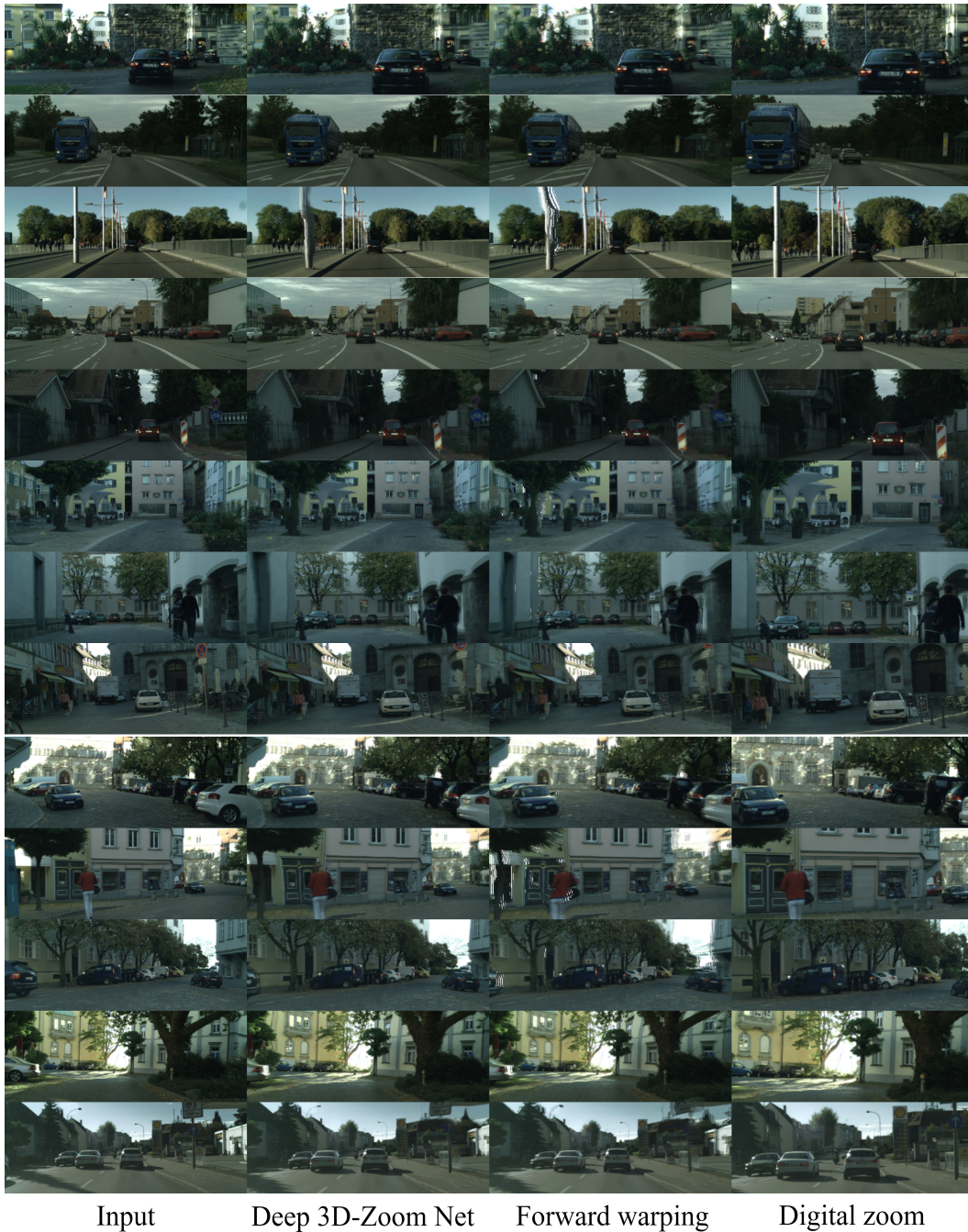
Figure 12: Subjective comparison on zoomed versions of the input images by three different methods for zoom factor 2.5. It is noted that the forward warping generates low-quality 3D-zoomed versions of the input image, while our Deep 3D-Zoom Net generates cleaner and sharper results with the input image’s structures well preserved.
