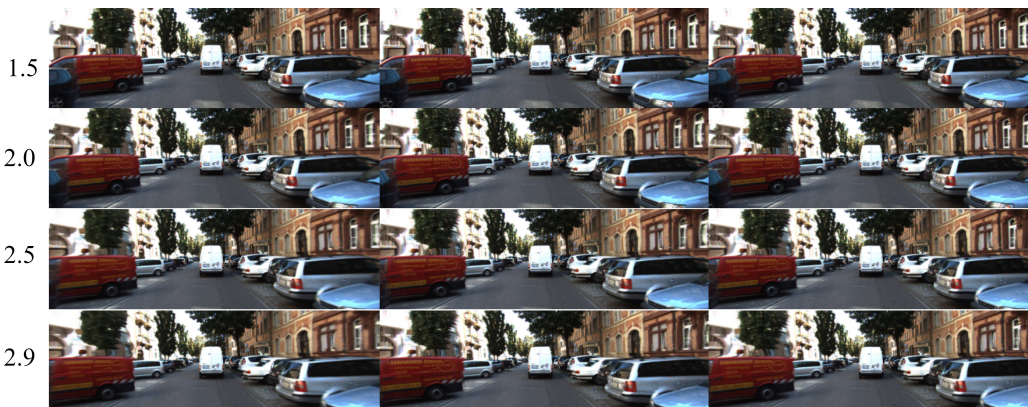
Figure 8: Results from ablation studies / NIQE score. A progressive improvement in terms of structure and sharpness can be appreciated from our model trained without perceptual loss to our model trained with perceptual loss and refinement block.
