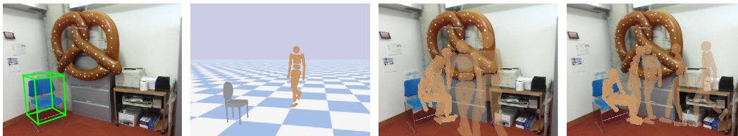
Figure 1: Synthesizing the motion of sitting. Left: Input image and 3D chair detection. Middle: Physics simulated environment for learning human-chair interactions. Right: Two examples of the synthesized motions.
