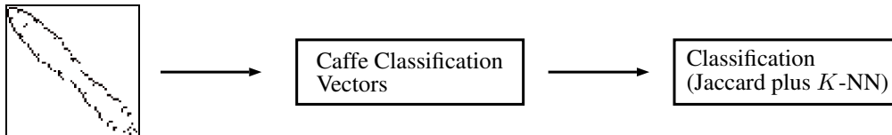
Figure 4: Classification of structured images using the classification vectors obtained from Caffe
