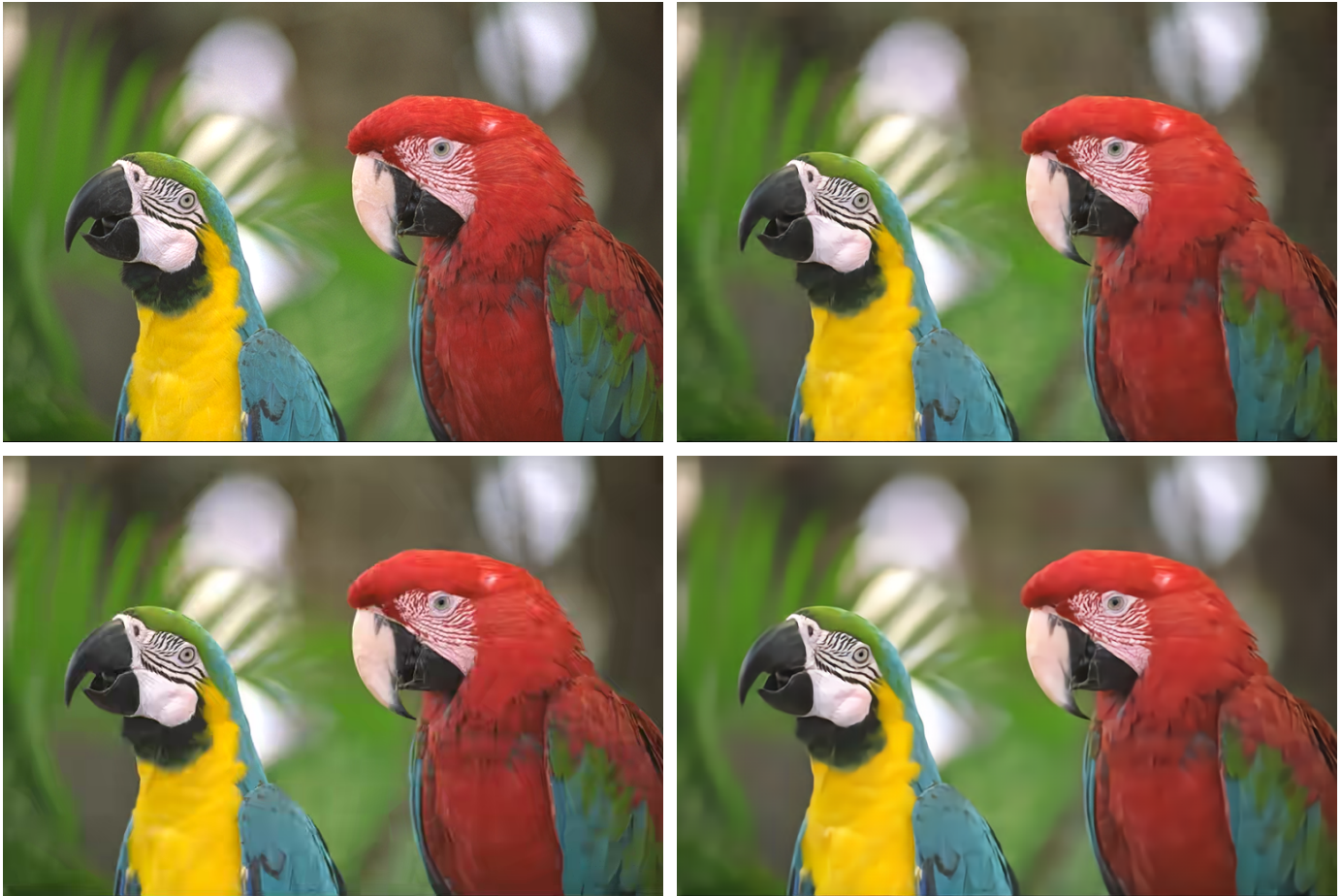
Figure 11: Sample test results. Top left, ground truth; top right, our method (MSE optimized; bpp, 0.1501; PSNR, 34.7103); bottom left, BPG (bpp, 0.1477; PSNR, 33.9623); bottom right, Ballé et al. (2018)'s approach (MSE optimized; bpp, 0.1520; PSNR, 34.0465)
