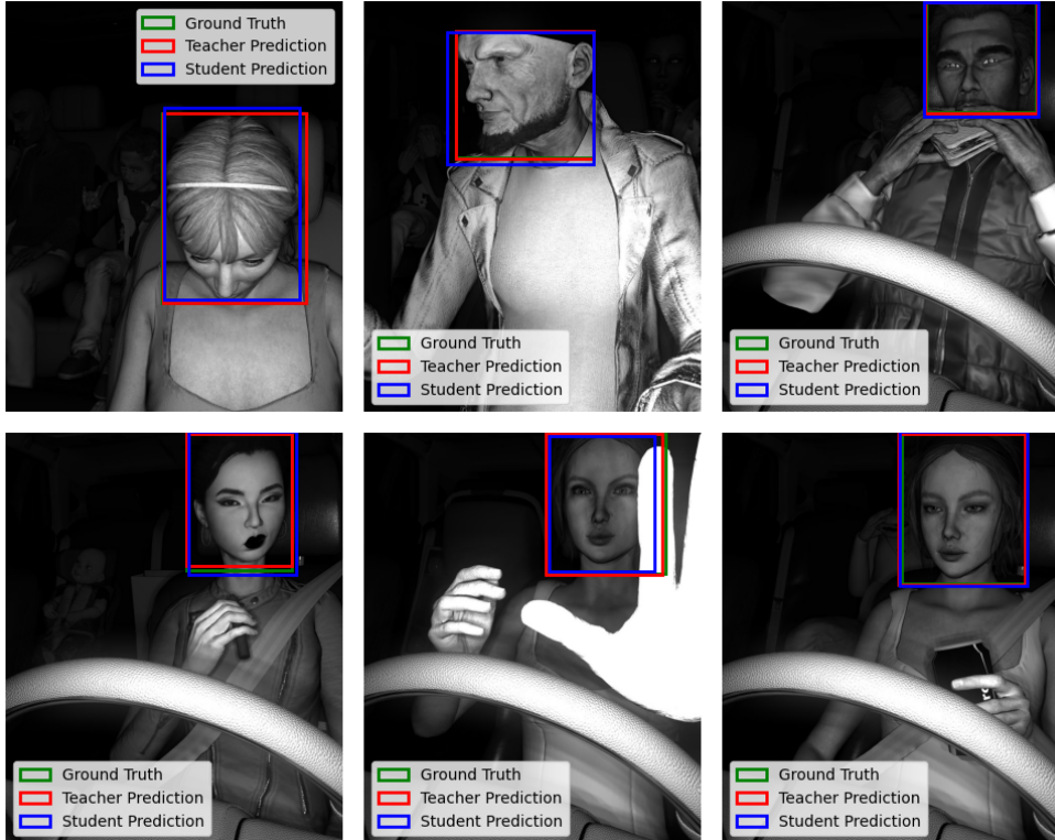
Figure 2: Example Bounding boxes of Driver’s face for Student, Teacher and Ground Truth
