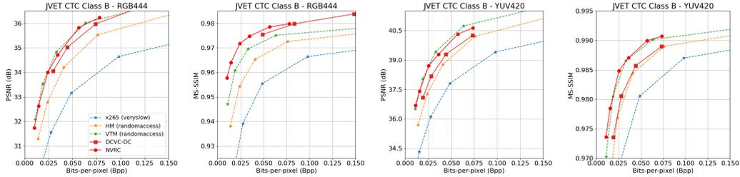
Figure 5: Average rate quality curves of various tested codecs on the JVET-CTC Class B datasets [9].
