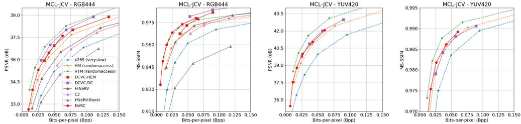
Figure 4: Average rate quality curves of various tested codecs on the MCL-JCV dataset [59].
