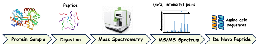
Figure 1: De novo peptide sequencing process using tandem mass spectrometry. Our goal is to predict amino acids sequence from the given spectrum as shown in the last two steps.
