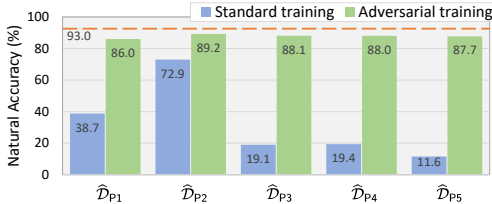
Figure 4: Natural accuracy on CIFAR-10 using VGG-16 under \ell_2 threat model. The horizontal line indicates the natural accuracy of a standard model trained on the clean training set.
