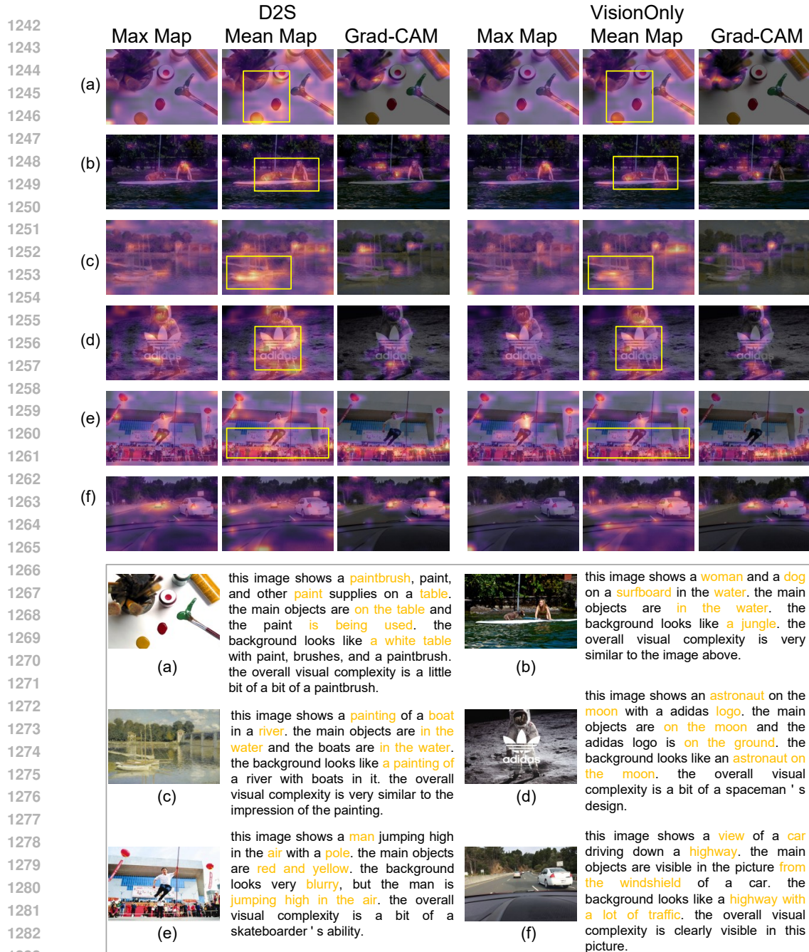
Figure 16: Feature activation maps. Visualization of channel activation maps (stage 4 in ResNet) using three approaches: maximum channel activation, mean channel activation, and Grad-CAM.
