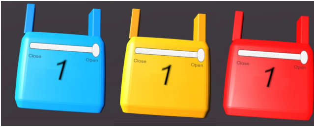
Figure 7: Fetch manipulation functional waypoints in the default state (left, blue), pre-check determined to be out of reach from the robot (middle, orange), and planner error (right, red)
