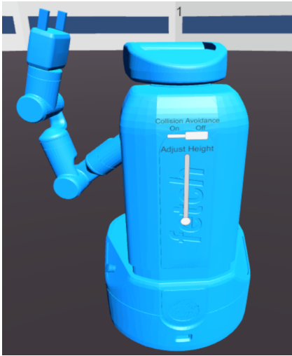
Figure 8: Example of a navigation functional waypoint for the Fetch robot including the Fetch robot model, a label indicating the functional waypoint’s order in the trajectory, a switch to enable or disable collision detection, and a slider interface to control the height of the robot.
