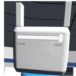
Figure 11: The operator can control the state of the robot's gripper through the slider interface on the virtual robot's end effector, however, unlike the functional waypoint the robot's state is immediately updated.
