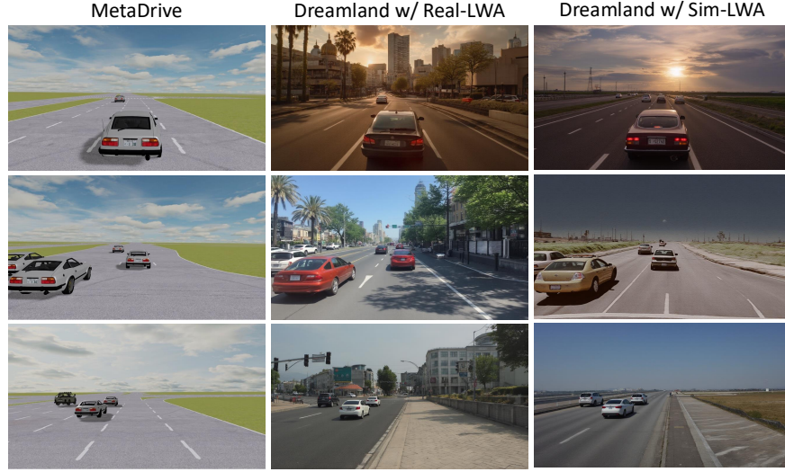
Figure 11: Ablation: Dreamland with Real-LWA and Sim-LWA. Dreamland using Sim-LWA as the Stage-3 input generates driving scenes with depth identical to the MetaDrive conditions, but loses fidelity to real driving scenes.
