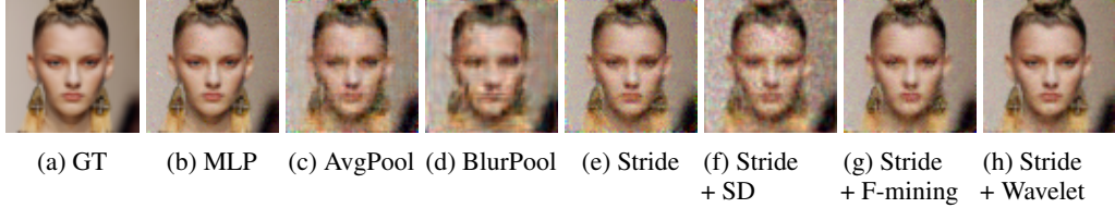
Figure 6: Reconstruction Guided by the Discriminator. All discriminators with downsampling lead to significant deviations from the ground truth. While F-mining and wavelets slightly improve the reconstruction, the spectral discriminator decreases image fidelity.
