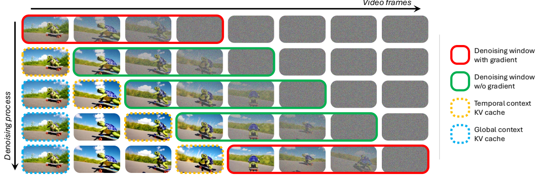
Figure 3: Illustration of the Rolling Forcing denoising process with T = 4 . Rolling Forcing jointly denoises a short window of consecutive frames that are assigned progressively higher noise levels and connected by bidirectional attention. The KV cache of recent frames is preserved as temporal context to maintain short-term consistency, while the KV cache of the initial frames is preserved as global context to ensure long-term consistency. During training, only a subset of denoising windows requires gradient computation, as highlighted by the red windows. These windows are mutually exclusive yet collectively cover all video frames.
