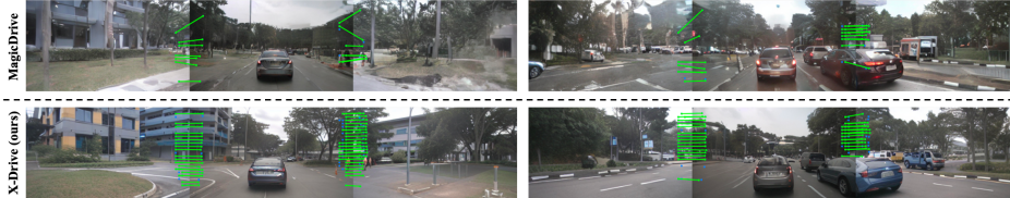
Figure 5: Key points correspondence between adjacent synthetic camera images. Our proposed method (bottom) can bring higher multi-view consistency than the baseline (top).
