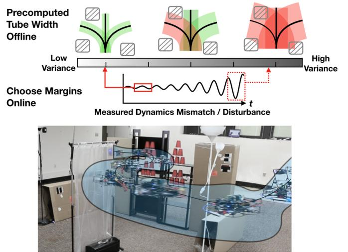
Fig. 1: **Adaptive Tube Library**: The proposed framework adapts safety margins online for a trajectory library with dynamics uncertainties estimated during flight to generate safe plans without overly sacrificing performance. To enable real-time adaptation, the library queries from a safety margin lookup table precomputed for each tube at discretized levels of dynamics variance.
