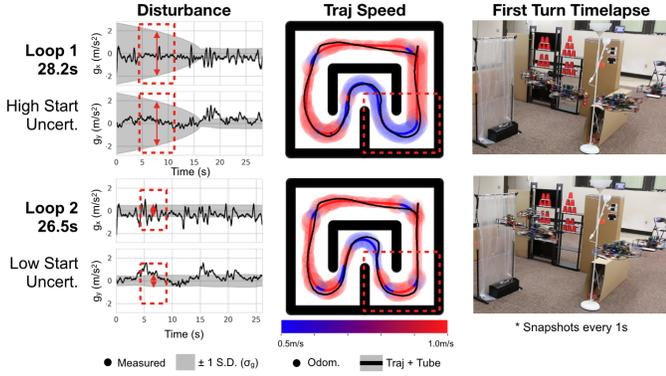
Fig. 2: **Exp. A - Higher performance with experience:** Safety margins adaptively decrease with lower uncertainty. At bottom-right corner, system picked the faster trajectory in the second loop when turning. Actual odometry (black) stays within tubes in both loops. Across two loops, average trajectory cost decreased from 0.249 to 0.218, and completion time from 28.2s to 26.5s.
