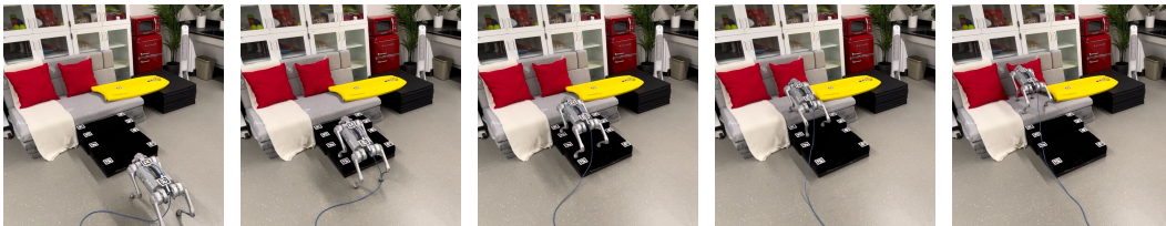
Figure 11: An illustration showcasing the robot’s climbing skill, the robot successfully ascends onto a sofa by navigating through box 1 and box 2 of differing heights.
