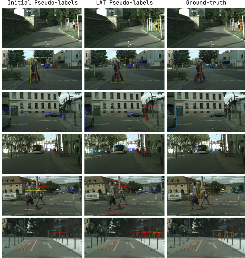
Figure 7: Qualitative results of nuImages target label space in class-divergent setting with Cityscapes dataset. Row 1: LAT detects an occluded pedestrian missed by initial pseudo-labels. Row 2: LAT corrects noisy human-annotated ground-truth. Row 3: LAT removes an erroneously predicted car from initial pseudo-labels. Row 4: LAT recovers a bus instance omitted by the upstream model. Row 5: LAT refines pedestrian bounding box and corrects its class label. Row 6: LAT recovers small-scale pedestrian and bicycle instances.
