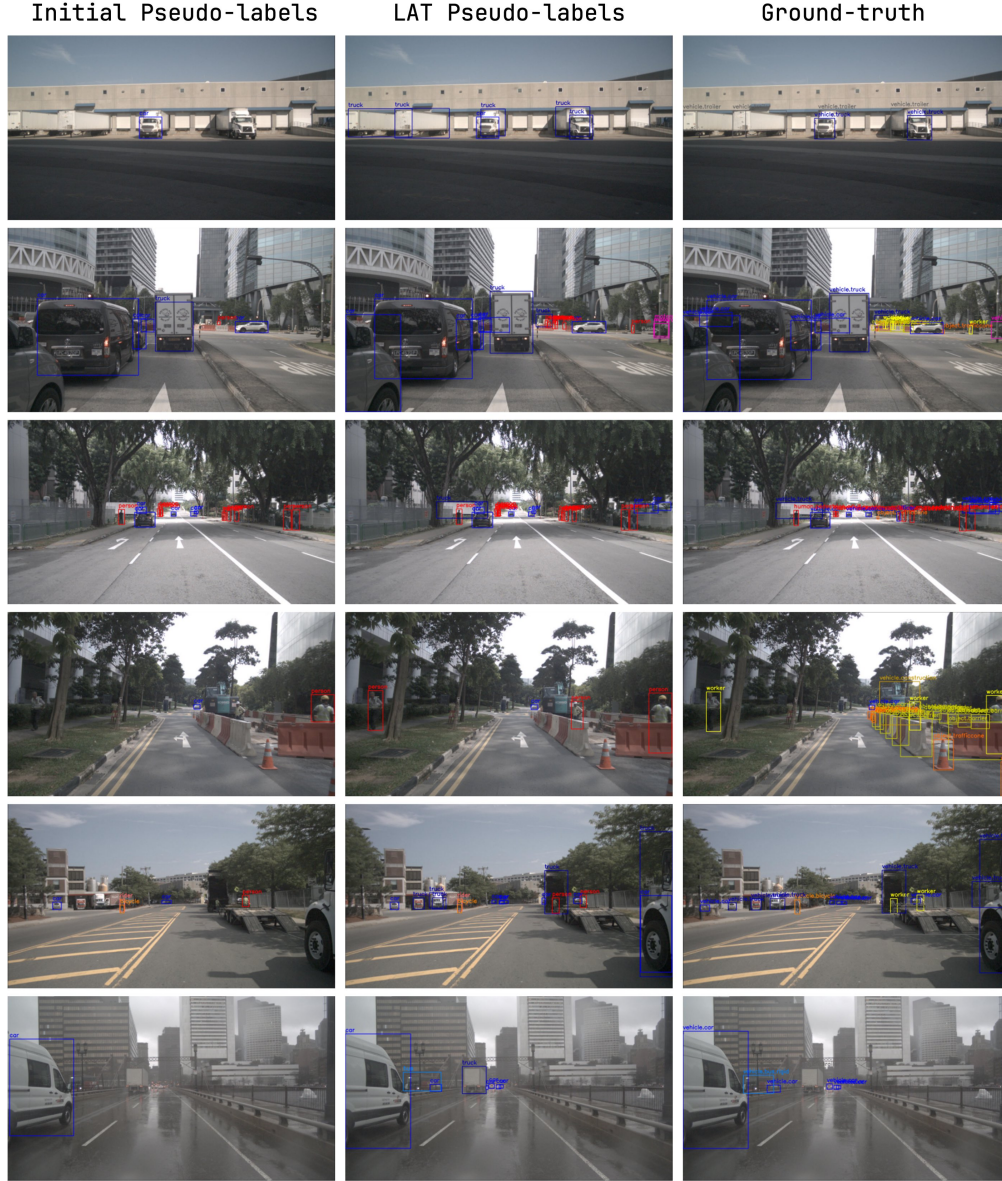
Figure 6: Qualitative results of Cityscapes target label space in class-divergent setting with nuImages dataset. Row 1: LAT recovers truck instances missing from initial pseudo-labels. Row 2: LAT refines truck bounding boxes and detects small objects. Row 3: LAT recovers heavily obscured cars. Row 4: LAT detects pedestrians omitted by upstream pseudo-labels. Row 5: LAT identifies foreground and background trucks. Row 6: LAT recovers vehicles under adverse weather conditions (rain).
