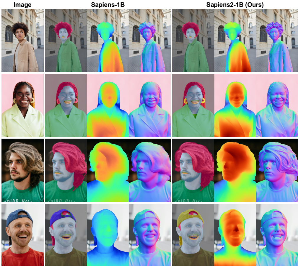
Figure 1: SAPIENS2 for dense-prediction tasks. We compare 1B models from both generations on segmentation, depth, and normals. Sapiens2 improves over Sapiens with stronger generalization and sharper segmentation of rare classes (lips, tongue, earrings), achieving pixel-accurate hair segmentation. On geometric tasks (depth, normals), it captures subtler facial, clothing, and hair details—all without task-specific architectures. post-training, we target fundamental human tasks—pose estimation (Zheng et al., 2023), body-part segmentation Thisanke et al. (2023), surface-normal (Bae & Davison, 2024), pointmap (per-pixel XYZ) (Wang et al., 2024) and albedo estimation (Ran et al., 2024). Relative to Khirodkar et al. (2024), we scale task-specific supervision by 10\times , typically on the order of 1M labels per task, and improve synthetic assets with more detailed geometry and photorealism. On the model axis, our largest variant has 5B parameters, accompanied by 0.4B, 0.8B, and 1B models for different compute settings and broader use. At a native resolution of 1K, our largest model achieves among the highest FLOPs reported for vision transformers. Fig. 1 showcases improvements over Sapiens for segmentation, depth and normals. Our models segment tiny accessories such as chains and earrings, and separate teeth and gums with pixel accuracy. Additionally, the predicted normals better capture facial wrinkles and hair details. Our evaluations show that learning at scale yields strong generalization across unconstrained human images and challenging in-the-wild conditions.
