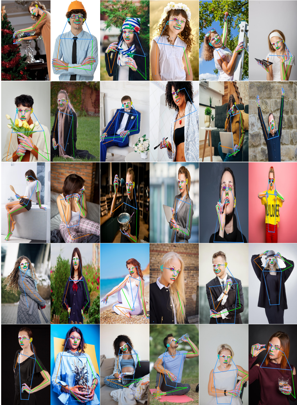
Figure 14: Top-down 308 keypoint predictions using Sapiens2-1B model on in-the-wild images.
