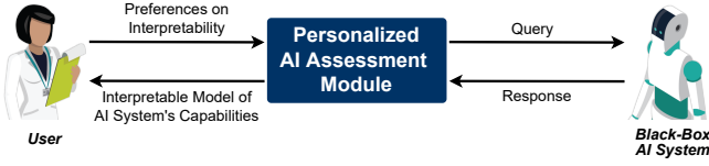
Figure 2: The personalized AI assessment module uses the user’s preferred vocabulary, queries the AI system, and delivers an interpretable model of the AI system’s capabilities.
