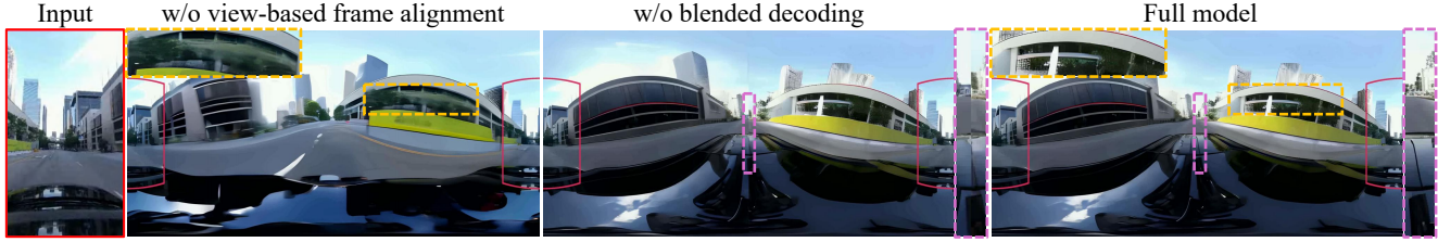
Figure 6. Qualitative ablation studies. The input region is marked in red. The 360° images are rotated 180° to illustrate the panoramic consistency. Compared to our full model, the variant without view-based frame alignment appears blurrier (orange box), while the variant without blended decoding shows artifacts in the center (pink box). Boxes are enlarged for ease of visualization.
