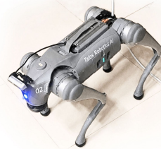
Fig. 1: A customized Unitree Go2 quadruped robot by Talos Robotics AI used for our real-world navigation experiments.
