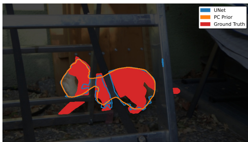
Figure 6. Ground truth annotations, baseline network prediction, and implicitly connected segmentation of one frame of the "cats05" sequence. In this case, the ground truth does not indicate a connected object - which contradicts our PC constraint. Accordingly, the prior with 57.8% IoU is inferior to the segmentation network (62.3%). Despite the IoU drop of 4.5%, it is application-dependent which of the segmentations are preferable.
