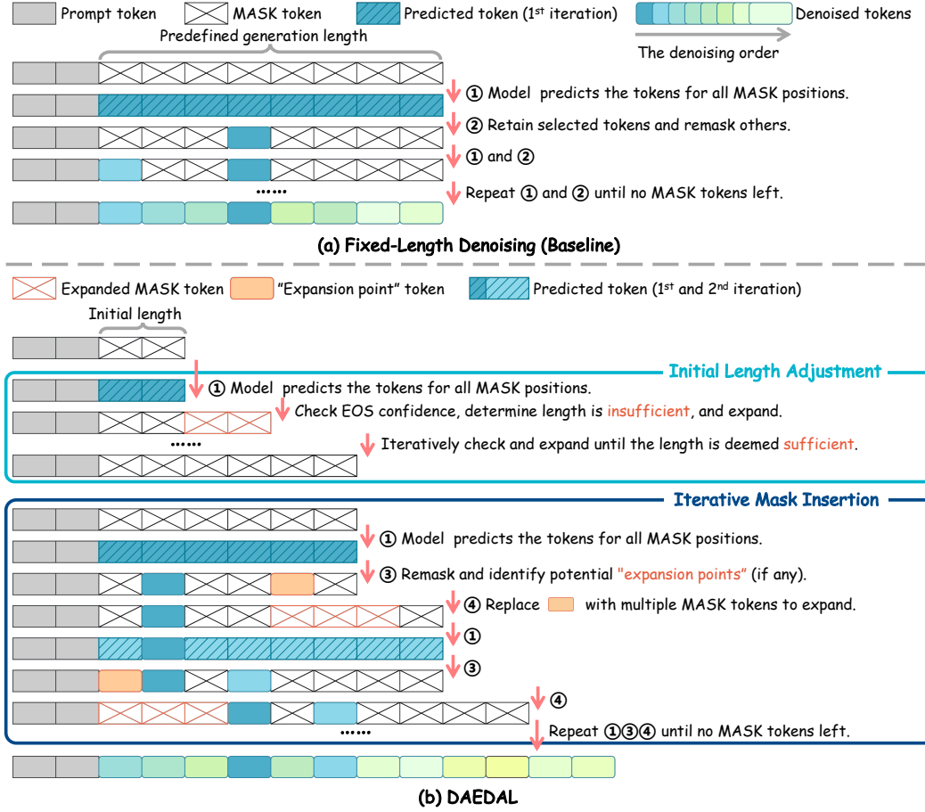
Figure 3: Inference process of Fixed-Length Denoising (Baseline) and DAEDAL. (a) The standard inference process for current DLLMs, which performs iterative denoising on a sequence of a predefined, static length. (b) Our proposed two-stage inference process, which first employs Initial Length Adjustment to determine an appropriate generation length before denoising, followed by Iterative Mask Insertion to expand the sequence on-demand during the denoising process.
