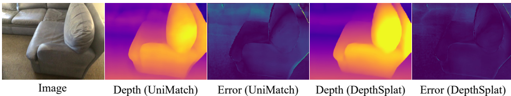
Figure 5: Depth Comparison on ScanNet. Our DepthSplat performs significantly better than UniMatch (Xu et al., 2023) on challenging parts ( e.g. , edges of the couch and pillows).
