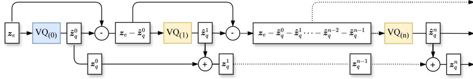
Figure 6: General RVQ architecture diagram for an arbitrary number of  $n$  residual quantizers.
