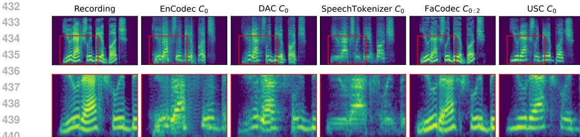
Figure 3: Spectrogram visualization of semantic  $C_0$  reconstruction of a speech sample from all the compared baselines, with a zoomed in view of the pitch harmonics. More examples in Appendix I.
