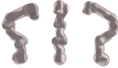
Figure 7: Illustrations of the Panda robot arm with capsule-shape collision primitives.
