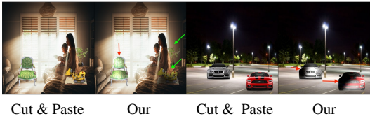
Figure 10: Failure Examples. The wrongly shaded regions are marked in red. In the first example, DIP aggressively copies background shading onto the chair. However, the lego and the plant are reshaded accurately. In the second, the reason for failure is surface normals. The scene has two dominant normal directions – ground (pointing upwards) and the sky (pointed towards viewer). The lack of third direction forces DIP to copy shading either from the sky or the ground plane.
