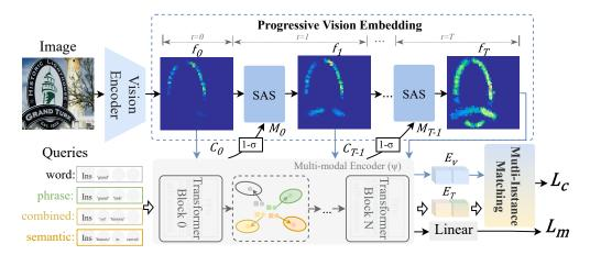
Figure 2: Overview of MSTAR. MSTAR is built upon four key components: a vision encoder  $\phi$ , the Progressive Vision Embedding (PVE), the multi-modal encoder  $\psi$ , and the multi-instance matching module (MIM). PVE incorporates image features  $f_t$  and the mask  $M_t$  derived from cross-attention map  $C_t$ , progressively shifting attention from salient features to fine-grained regions.
