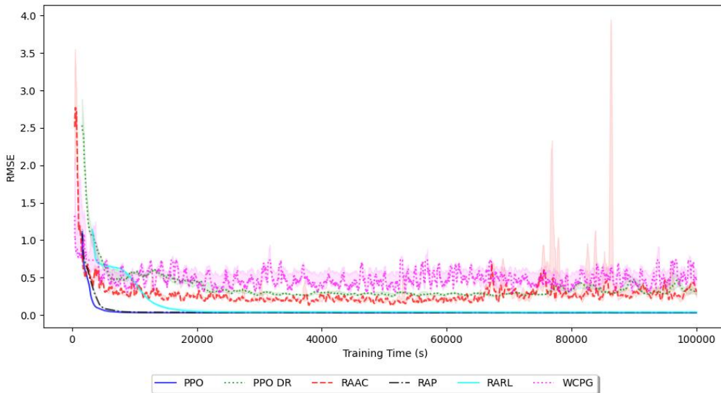
Figure 11: Learning curves of the RL agents and robust baselines on the quadrotor tracking task.
