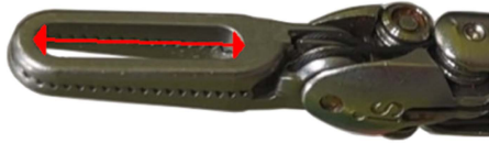
Fig. 8. Image of the da Vinci Cadiere Forceps, with the lumen length dimension (as we name it) indicated with a red arrow.
