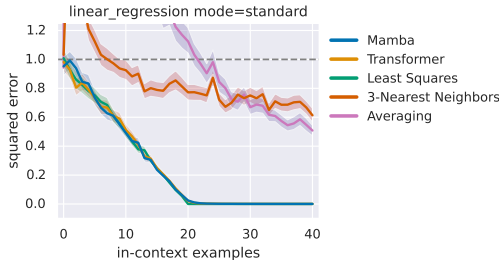
Figure 7: Mamba compares with transformers when trained and tested on the same unskewed linear regression task distribution. We report one training run for each plot and method
