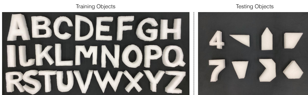
Figure 16: Push-Shape Objects. The training set includes all 26 capital letters of the alphabet, while the testing set consists of 8 shapes, including digits and polygons.
