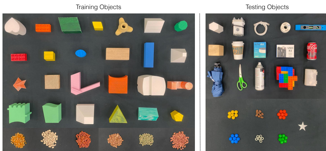
Figure 15: Sweeping Objects. The training set includes 25 distraction objects and 6 colored beans, with 5 to 6 distractions in the scene at a time during data collection. The testing set includes 15 real-world distraction objects and 6 colored particles. The star is used as the target in the experiments.
