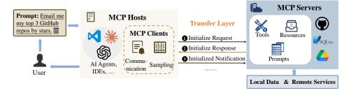
Figure 1: Overall architecture and workflow of the MCP-powered agent system.
