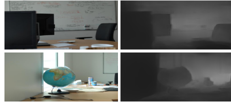
Figure 7: Further verification on realistic scenes from DSLR dataset. First column: Input real defocus images; Second column: Predicted depth maps from DefocusNet. Our model can also work well in real scenes with real defocus blur.
