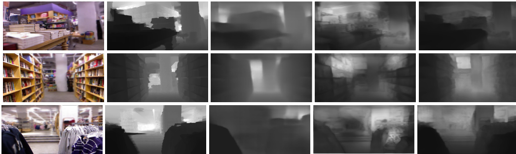
Figure 5: Visual comparison between our method (trained on the synthetic dataset) and other recent single-view depth estimation methods (fine-tuned on the synthetic dataset). Left to right: Input defocus image at the focal plane of 1 meter; Ground truth depth map; Predicted depth map from Laina et al. (2016); Predicted depth map from Alhashim & Wonka (2018); Our output from DefocusNet. Brighter color represents a farther distance.
