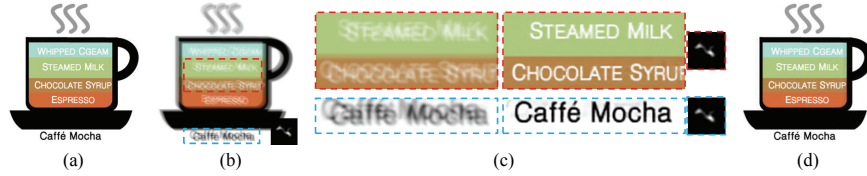
Fig. 10. Deblurring of a blurred image with different text regions. (a) ground truth image, (b) synthetic blurred image and its kernel, (c) cropped images of (b) and our deblurring results, (d) final deblurring result of (b).
