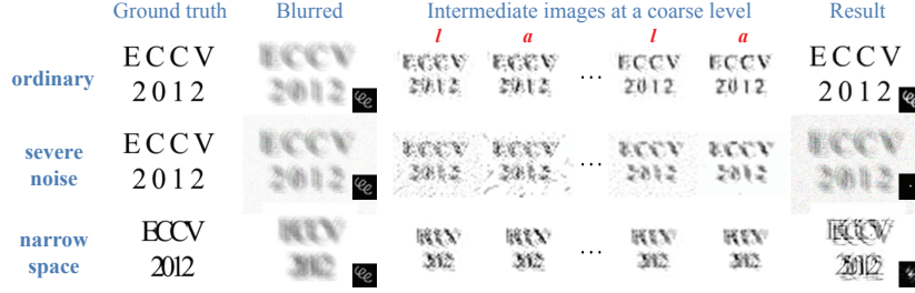
Fig. 7. Failure cases. (top row) our intermediate and final results on a synthetic example; (middle row) results with added severe noise; (bottom row) results with narrow spaces between characters.
