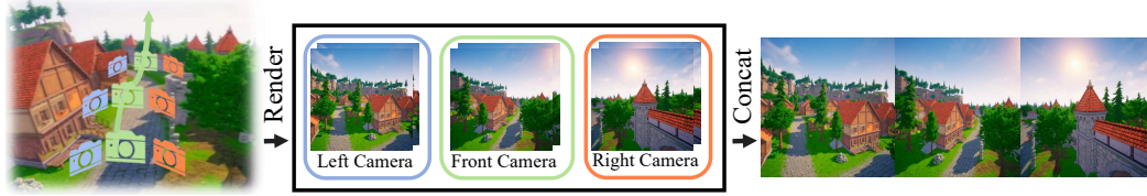
Figure 5: The overview of ConsistView. It first renders overlapping multi-view images, then concatenates them into a unified video for consistent restoration.
