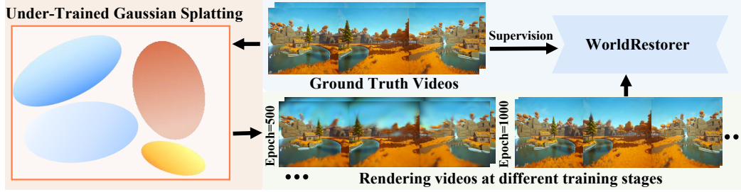
Figure 3: The overview of the training WorldRestorer. An under-fitted Gaussian Splatting model is trained using ground truth videos to render degraded videos at different training stages, which are paired with corresponding GT videos for training WorldRestorer.
