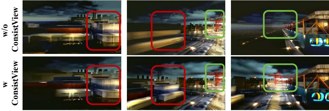
Figure 8: Visualization comparison of WorldRestorer with and without ConsistView. The first, second, and third columns correspond to the left, front, and right views, respectively. Overlapping regions between views are indicated by the red and green boxes.
