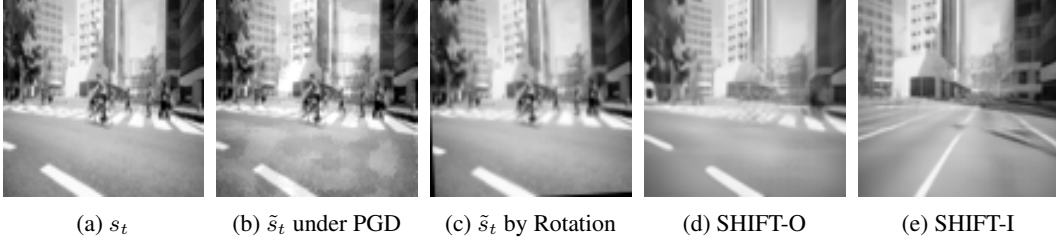
Figure 2: Examples of true and perturbed states captured by the front camera of a vehicle in the AirSim driving simulator. a) is the true state. b) and c) are the perturbed states under the PGD attack with a l_\infty budget of \frac{15}{255} and through rotation [31] by 3 degrees counterclockwise, respectively. d) and e) are the perturbed states generated by our SHIFT-O and SHIFT-I attacks, respectively. Neither PGD nor Rotation attacks can alter the decision-related semantics. SHIFT-O removed pedestrians and bicycles at the crosswalk while being aligned with the real history. SHIFT-I lures the driver into thinking that the car has already crossed the crosswalk, when in fact it has not in the real environment. Note that SHIFT-I is history-aligned with the observed trajectory but not the real trajectory.
