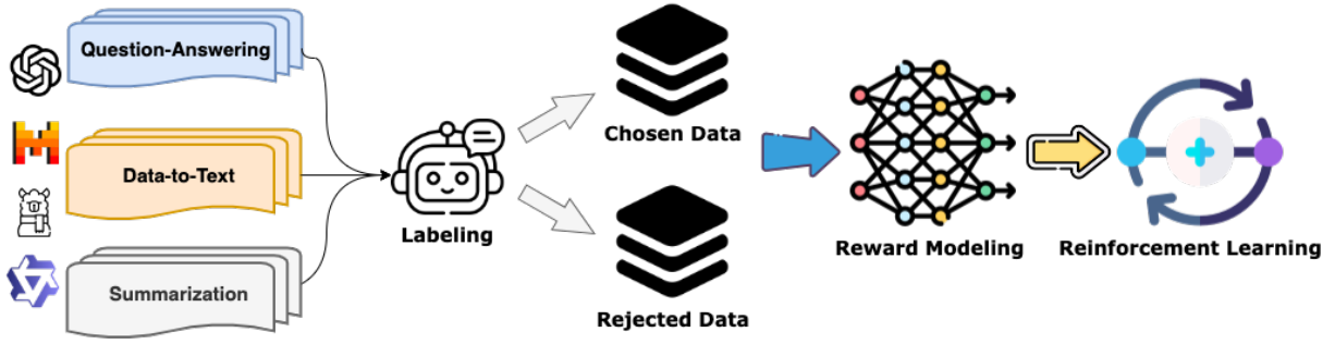
Figure 1: An overview of our data labeling method and our experiments based on the preference data in RAG Scenario. We use o3-mini as the judge to evaluate the quality of the generation from multiple models. We then train the reward models and use them for Reinforcement Learning.
