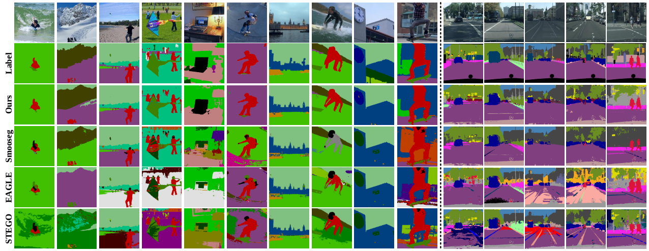
Figure 4: Quantitative comparison of the results of the proposed IL2Vseg and other state-of-the-art methods on the COCOStuff (left) and Cityscapes (right) datasets.
