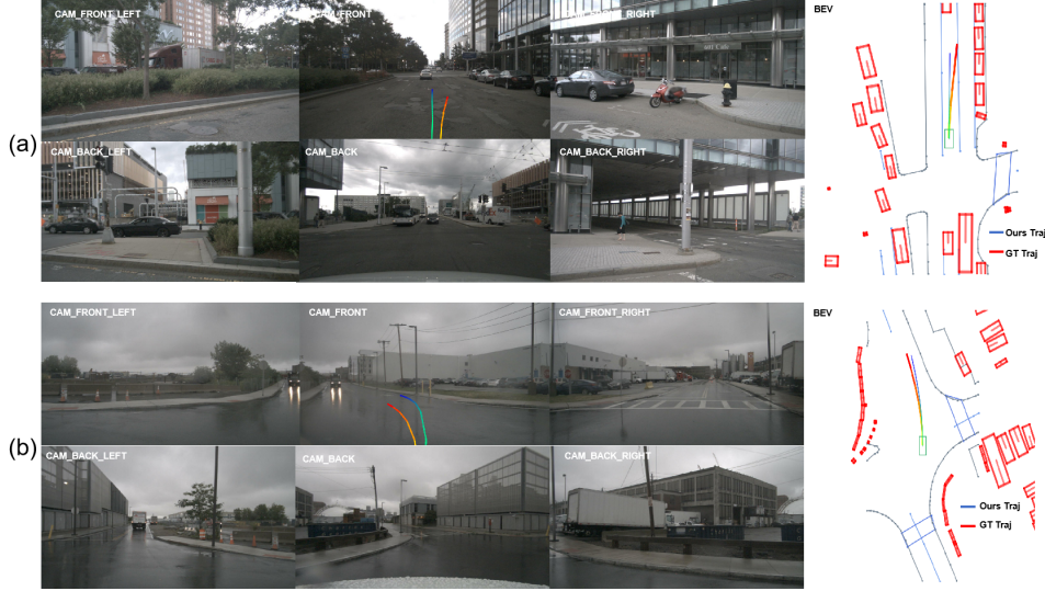
Figure 4: Visualization of failure cases. We highlight two distinct planning failure cases. The first arises when the navigation cue in the ground-truth annotation is ambiguous, and the second occurs in open spaces where the predicted trajectory deviates during a turn. In each figure, the green icon denotes the ego vehicle, while red icons mark surrounding vehicles and other dynamic objects.
