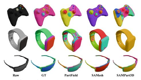
Figure 4: **Part Segmentation Results on PartNeXt**. PartField struggles to separate connected regions, SAMesh excels at fine-grained segmentation but over-segments, while SAMPart3D lacks continuity in weak textures and granularity control.
