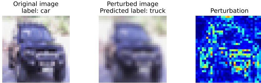
Figure 3: Comparison between Original and Perturbed Images using Gaussian blur attack. Left: Original Image with True Label car , Center: Adversarial Image with Predicted Label truck and Right: Perturbation
