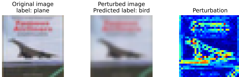
Figure 4: Comparison between Original and Perturbed Images using Gaussian blur attack. Left: Original Image with True Label plane , Center: Adversarial Image with Predicted Label bird and Right: Perturbation
