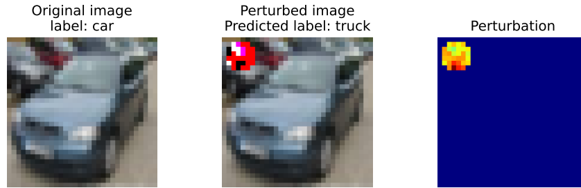
Figure 5: Comparison between Original and Perturbed Images using Patch attack. Left: Original Image with True Label car , Center: Adversarial Image with Predicted Label truck and Right: Perturbation
