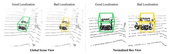
Figure 2: Example *Car* objects converted into normalized box view (NBV). Foreground/background points are marked in black/gray, respectively for better visualization. Foreground LiDAR points distributing tightly within a  $[-1, 1]^3$  NBV cube is a domain-consistent sign for good localization.
