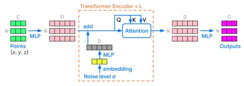
Figure S7: Architecture overview of DiffuBox's denoiser model. The model is composed of 2 MLP layers and L transformer encoder layers, which maps 3D points to a higher dimensional space for effective self-attention.
