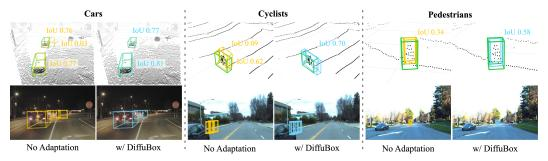
Figure S10: Additional Qualitative Results of DiffuBox for other classes. We include additional visualizations of 3D object detection for different classes. We color the ground truth boxes in green, the detector outputs in yellow, and the boxes refined with DiffuBox in blue.
