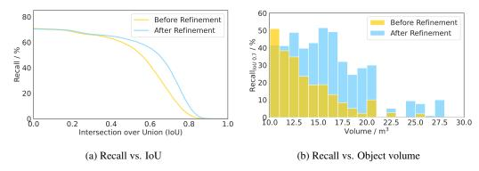
Figure 6: **Recall improvement with DiffuBox.** We report recall on the *car* class (KITTI  $\rightarrow$  Lyft, PointRCNN) before and after refinement with DiffuBox.
