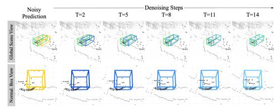
Figure S8: **Box refinement through denoising steps.** We visualize the correction of a noisy prediction, shown in yellow, using DiffuBox, as well as the normalized box view. The detection output is refined iteratively though the denoising steps, resulting in the final, corrected output of our method.
