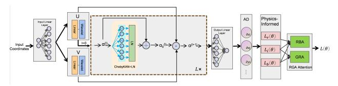
Figure 1: Architecture of the complete AC-PKAN model. It combines its internal attention architecture with an external attention strategy, yielding a weighted loss optimized to obtain the predicted solution.
