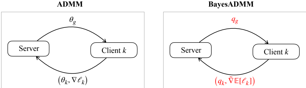
Figure 1: In ADMM, the server broadcasts the global parameter \theta_g to the clients who then update their local \theta_k and send them back to the server along with the gradients \nabla \ell_k of their loss functions. Bayesian-ADMM generalizes ADMM by using distributions over global and local parameters (denoted by q_g and q_k , respectively) and replacing gradients by natural gradients (denoted by \tilde{\nabla} \mathbb{E}[\ell_k] ).
