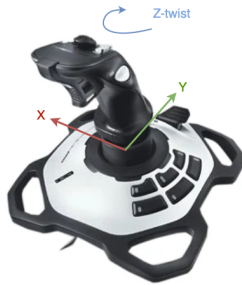
Figure 9. Extreme3D Pro Joystick & Co-ordinate System
