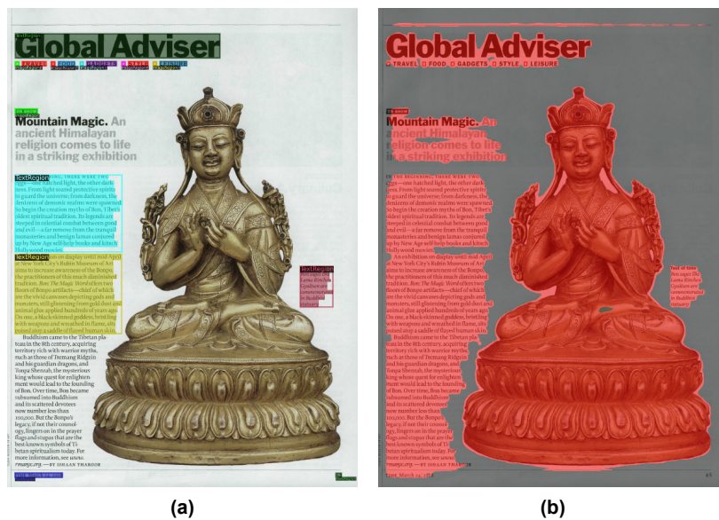
Figure 9: Result of a typical magazine image from PRIMA dataset using our learning technique. (a) The real annotation provided for the document. (b) The predicted mask generated using our proposed learning technique with AutoDocSegmenter-MNV3sm. Our proposed method have been able to outline the complex boundary of the image while it is kept non-annotated in the given dataset.
