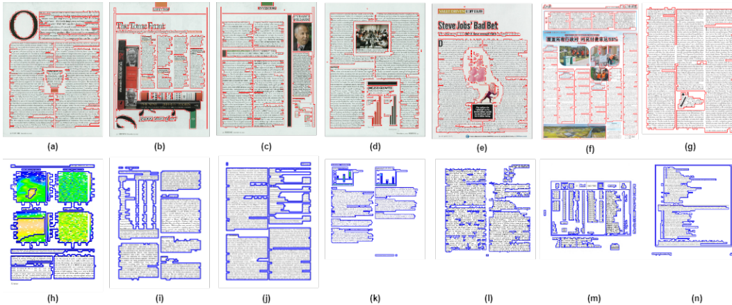
Figure 4: Annotating documents using isothetic covers. (a)-(e) Results from PRImA dataset, (f)-(g) Results from M 6 -Doc dataset, (h)-(j) Results from PubLayNet dataset, and (k)-(n) Results from DocLayNet . The algorithm is able to annotate complex layouts of in-line images, tables, circuits and graphs.
