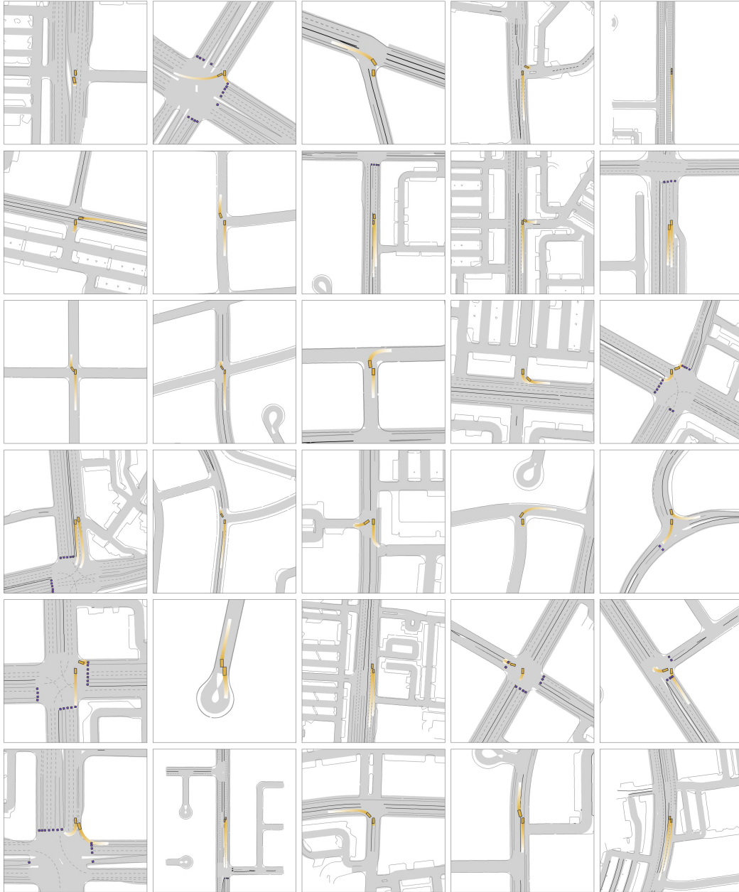
Figure 8: Various safety-critical layouts from DIVA-Sim. The yellow rectangular represents the ego-car and the other cars interacting with it. All scenarios are initialized by the Waymo Open dataset [65] and generated by adversarial interactions [80] within simulators.
