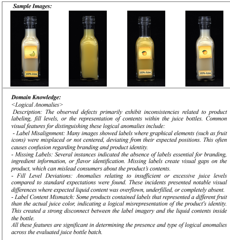
Figure 17: A case of domain knowledge. Domain knowledge includes descriptions of defects. In this example, the text outlines four major logical anomalies that may occur in these juice bottles. The actual dataset contains some rare logical anomalies that are not described, such as the incorrect icon placement in the first image. We do not expect domain knowledge to cover all possible anomalies; its primary role is to provide MLLMs with an understanding of the types of anomalies.
