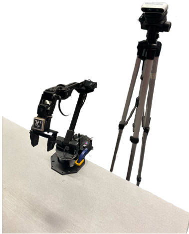
Figure 7: Our WidowX hardware setup includes a 6-DOF Trossen Robotics WidowX 250 S arm attached to a table with a 2-fingered gripper and an Intel RealSense Depth Camera D435.
