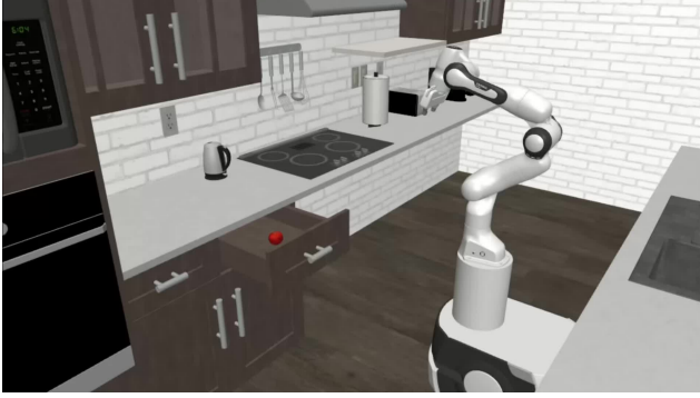
Figure 9: Our RoboCasa simulation setup includes a 7-DOF Franka Emika Panda arm with a 2-fingered gripper.
