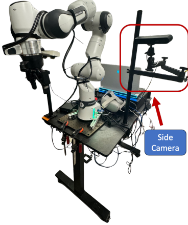
Figure 6: Our Franka hardware setup includes a 7-DOF Franka Emika Panda arm with a Robotiq 2-fingered gripper and a Zed 2 stereo camera mounted on the base.
