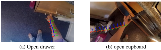
Figure 4: 6D wrist post-grasp policy outputs on unseen images. The red, green, and blue arrows denote the x, y, z coordinates of the wrist orientation in the camera frame.
